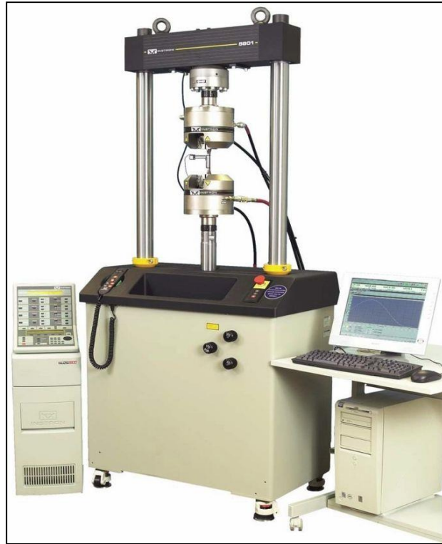
Figure 141 Closed-loop Servohydraulic test system including personal computer [74].
